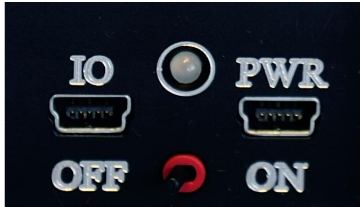
Fig. 2 Interface (IO) and power (PWR) connectors of the labZY Tools.
