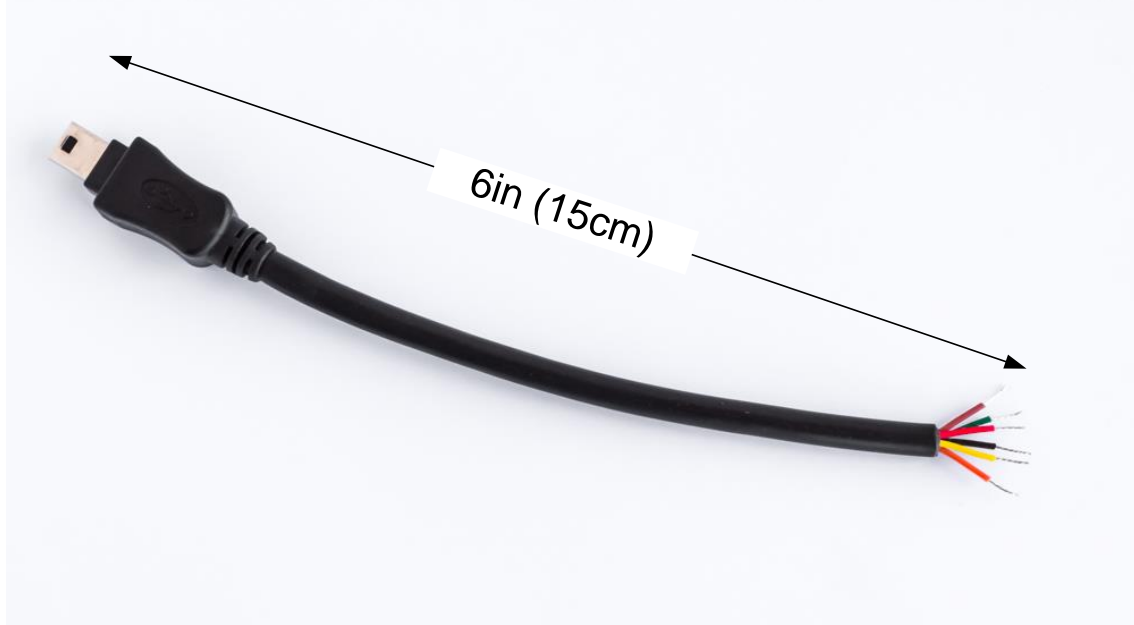
Fig 3. Cable for connecting the labZY Tools directly to UART ports.
