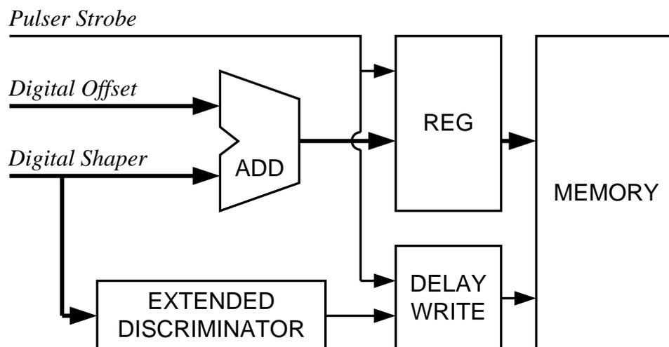
Fig. 2 Block diagram of digital pulser.
