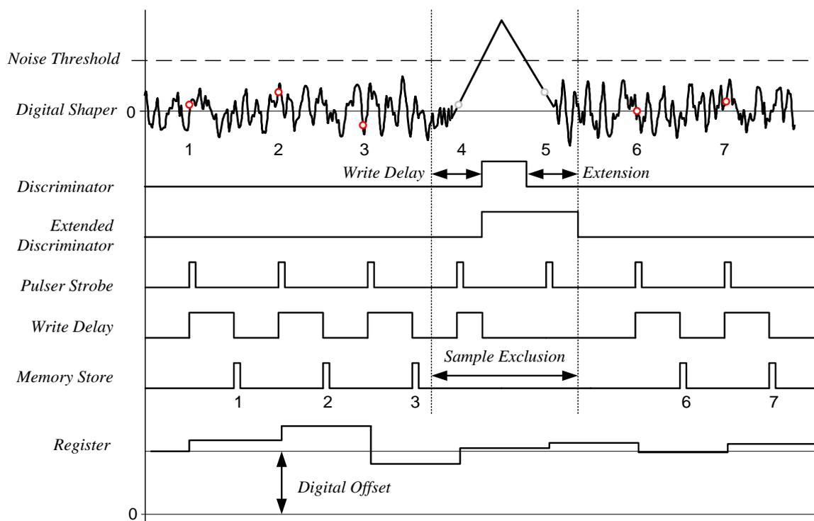
Fig. 3 Timing diagram illustrating the digital pulser operation.
