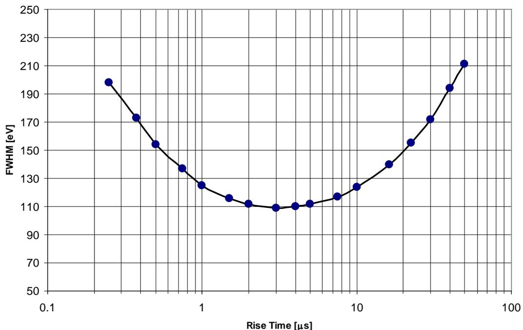
Fig. 5 Electronic noise profile of digital spectroscopy system.
