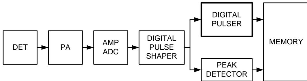
Fig. 1 Simplified block diagram of digital spectrometer using digital pulser.
