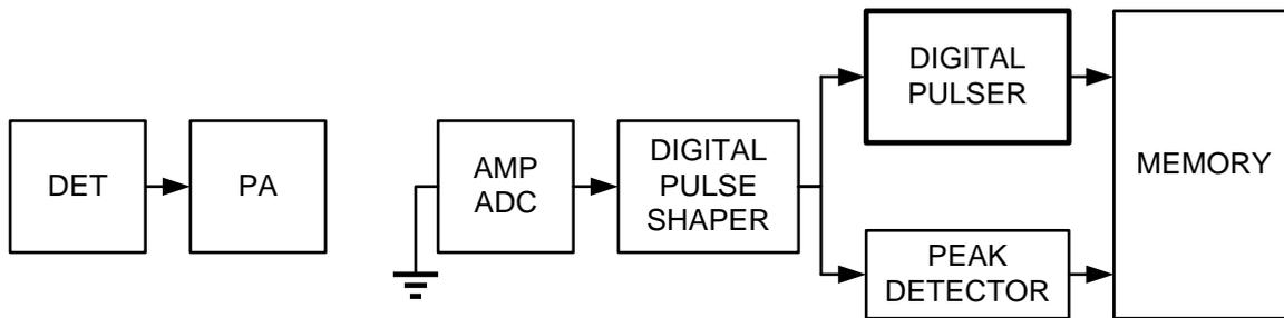
Fig. 6 Test configuration excluding detector and preamplifier from the signal processing chain.
