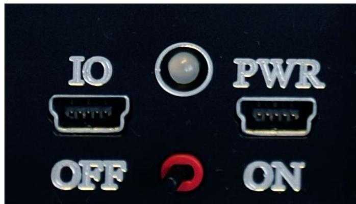
Fig. 2 Interface (IO) and power (PWR) connectors of the labZY Devices.
