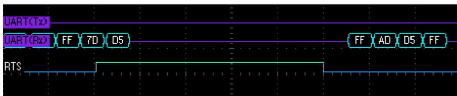
Fig. 6 Pausing data flow using the RTS line.
